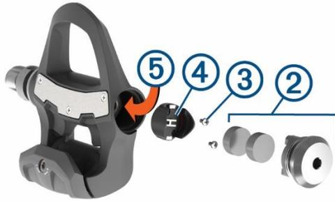
5. Use a small Phillips screwdriver (PH 00) to remove the two screws (3) from inside the battery carriage (4).
